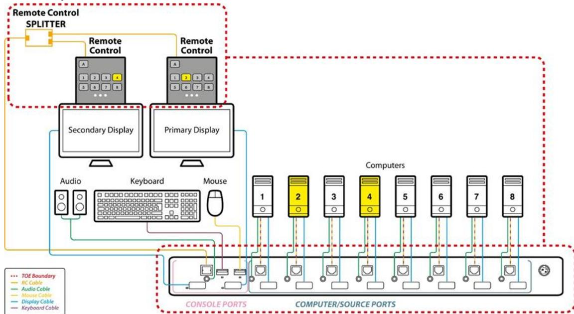
**Figure 2: – Evaluated Configuration for Combiner Switches.**
